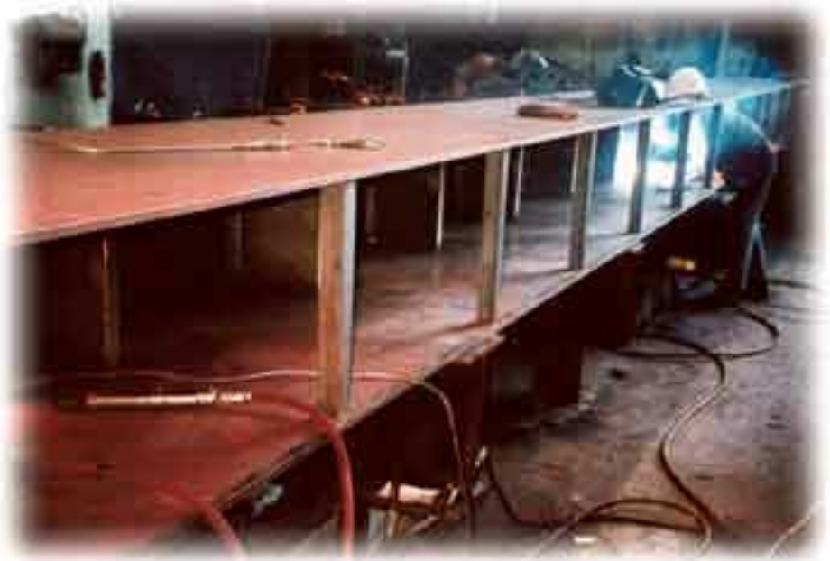
Figure 2. Fabrication of the pile cap. Angle braces were welded to the base of the webs to minimize distortion/warpage and to support the bottom flange during fabrication.
