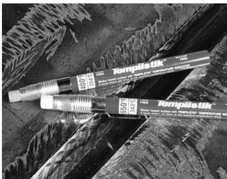
Figure 2. Tempilstiks™ help control interpass temperature.
