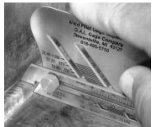
Fillet weld sizes can be measured with gages. (Photo courtesy of G.A.L. Gage)
