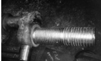
Figure 13. Shaft repaired using spread arc technique.
