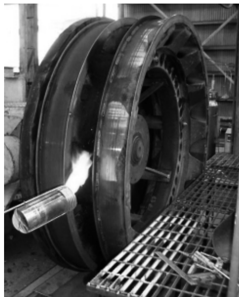
Figure 6. Preheat of massive part.
