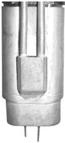
Figure 3. The tandem torch permits the delivery of two electrodes: the lead arc and the trail arc. The nozzle provides uniform shielding gas coverage for the molten weld pool.
