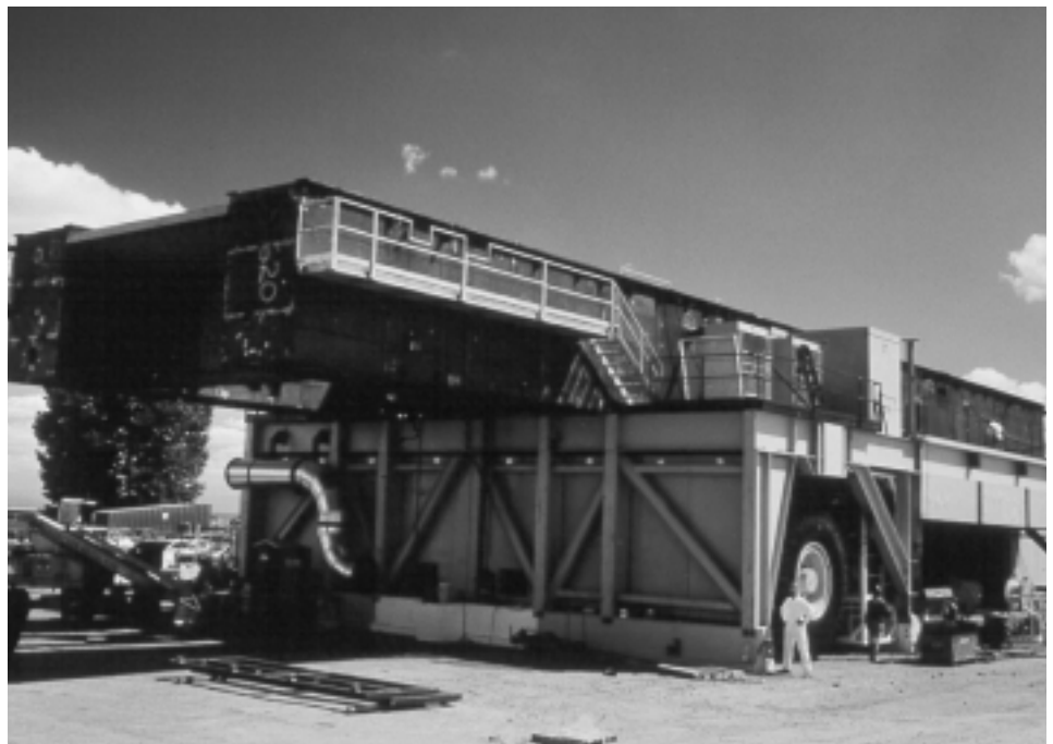
Figure 2. First test drive of the completed substructure. Box beams cantilever from the rear end of the rig.
