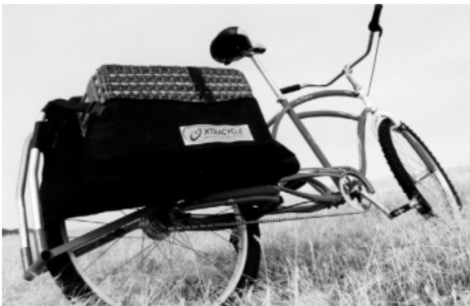
Figure 2. The modular, TIG-welded FreeRadical™ model is intended for use primarily in developed countries.
