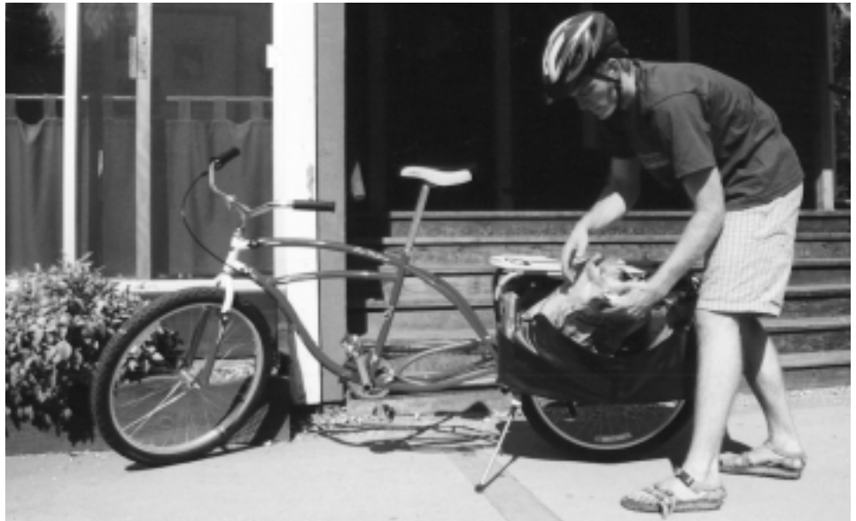
Figure 1. The Xtracycle can turn virtually any existing bicycle into a load-carrying vehicle.
