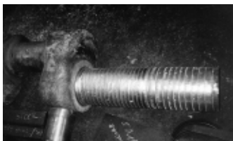
Figure 13. Shaft repaired using spread arc technique.
