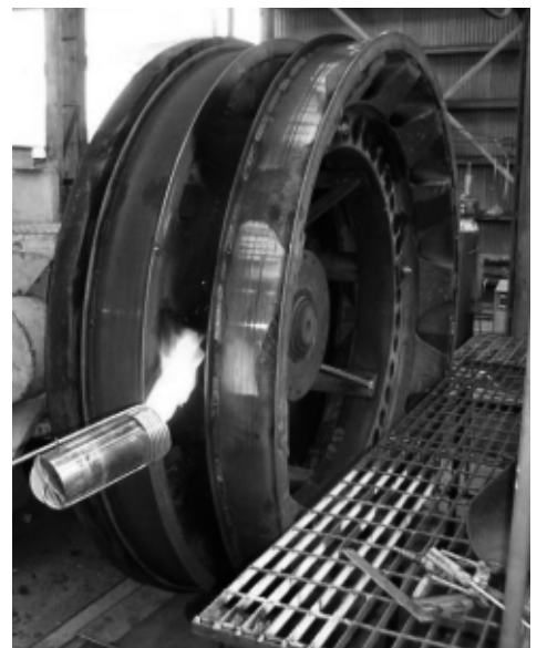
Figure 6. Preheat of massive part.
