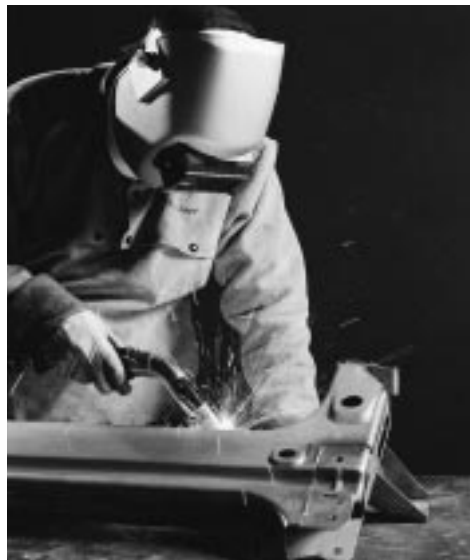
Figure 10. "After" - welding with fume removal gun.
