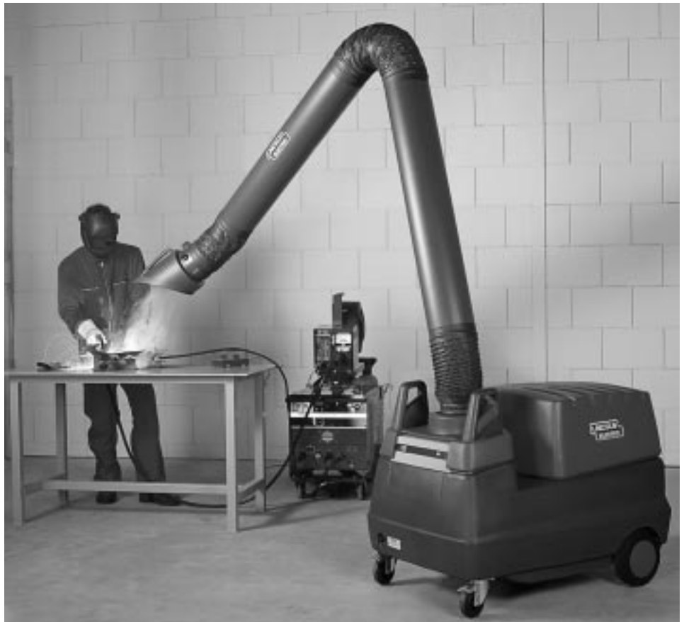
Figure 4. Low vacuum/high volume system (mobile unit).
