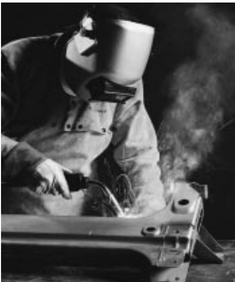
Figure 9. "Before"- welding without fume removal gun.
