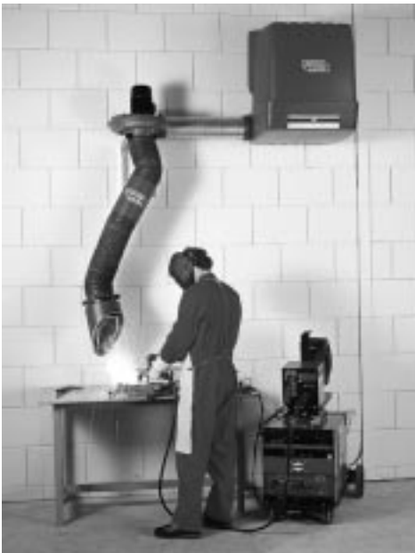
Figure 3. Low vacuum/high volume system (wall mount).
