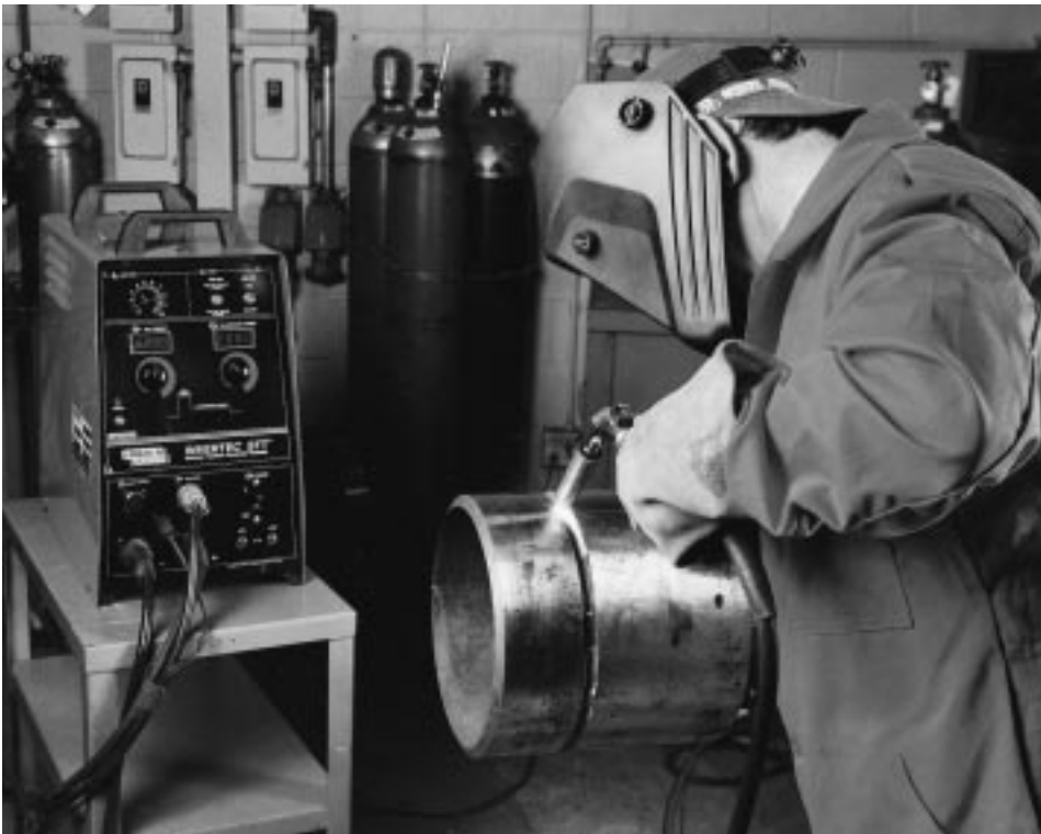
Figure 2. Invertec STT®, shown here in a pipe welding application, greatly reduces fume generation.
