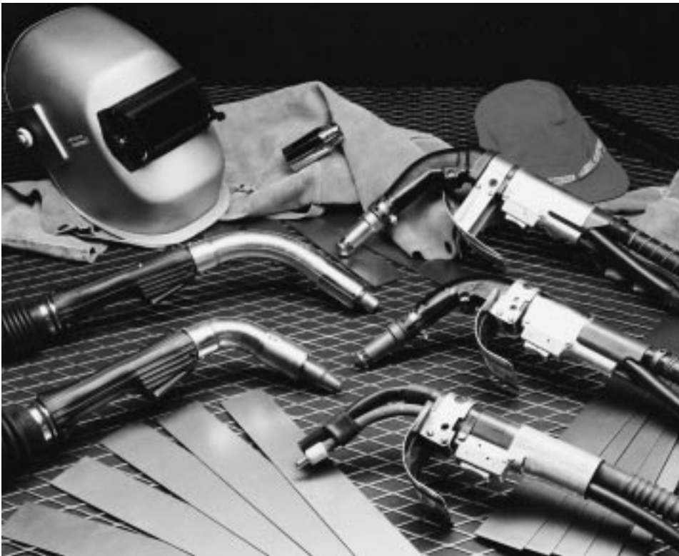
Figure 8. Examples of high vacuum/low volume welding guns.
