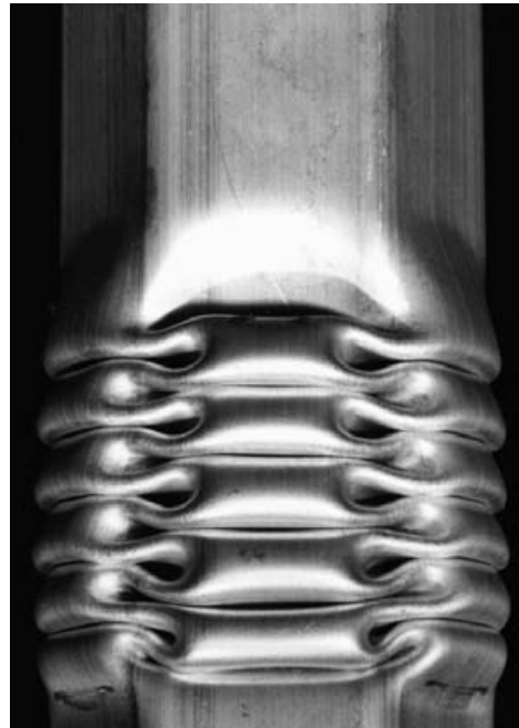
Figure 1. Aluminum front frame rail crushed in crash test showing uniform crushing and energy absorption.
