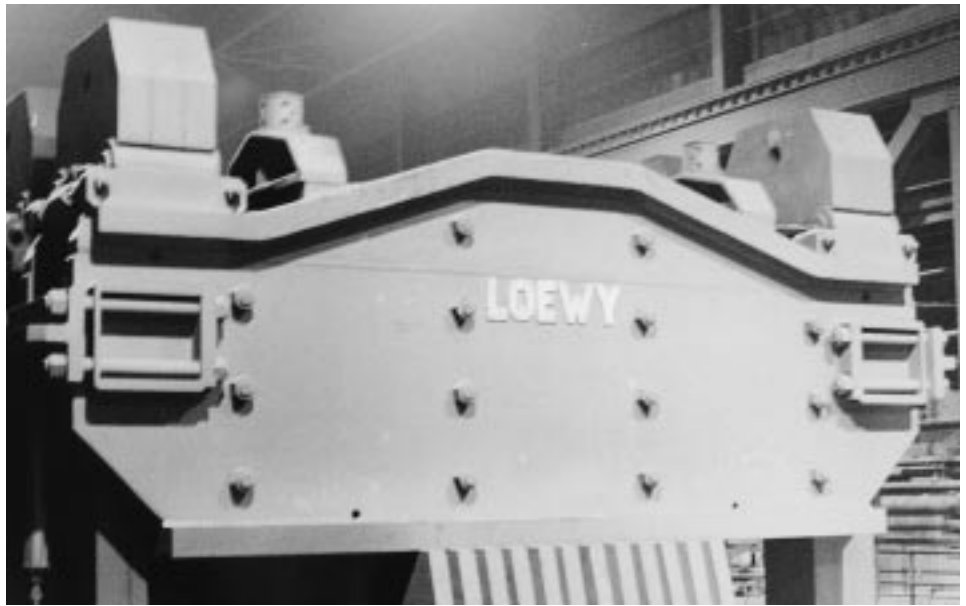
Figure 5. 50,000 ton (50,803 m ton) Loewy forge press grinder.
